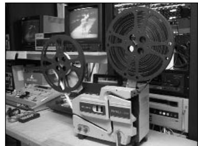
Some budget-minded repositories make low-cost videotape access copies in-house using an Elmo film-to-tape transfer unit.
