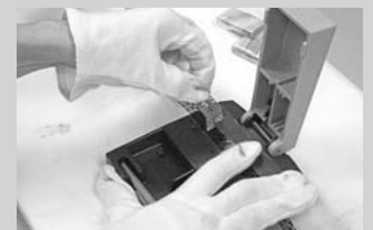
Photographs, contributed to the guide by George Eastman House, illustrate common film formats and safe handling practices. This sequence shows how to make a splice using presstape.
